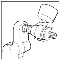
Place the swivel arm of the kitchen machine vertically, press the grain mill with mount onto the machine in such a way that the tangs engage into the grinding shaft in the drive section.
