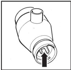
In order to avoid a defect in your kitchen machine when the grain mill is overloaded, the grinding shaft (2) has been provided with a predetermined breaking point, which breaks when it is overloaded approx. three times.
